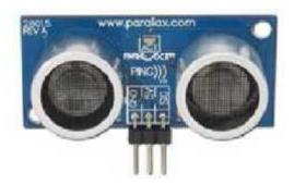
Gambar 2.12 Sensor jarak ultrasonik ping
